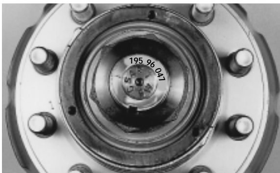
Identification of axles without type plate Production No. of axle on right of axle tube as seen in direction of forward travel
