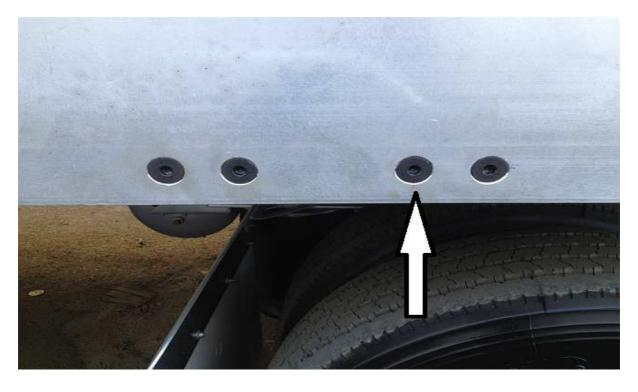
Torque Nyloc nut on the CSK Cap screws as indicated by arrow above to 108 NM periodically every 50,000 km
