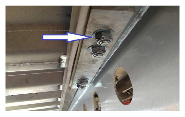
Torque all bolts as indicated by arrow above on clamp plates to 148nm periodically every 50,000 km
