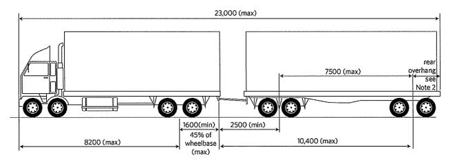
Note 1: Axle sets may be replaced with alternative axle sets at the same axis points Note 2: Maximum rear overhang is the lesser of 4300mm or 50% of the forward distance
